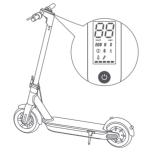
1. Power on the KickScooter and check the power level indicator. Charge the KickScooter if the battery level is low.
