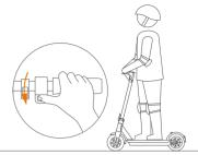
Put your other foot on the footrest to keep both feet stable. Press the throttle on the right hand to speed up when you are balanced.
